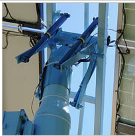
A 1998 model of a passive solar tracker, viewed from underneath.
