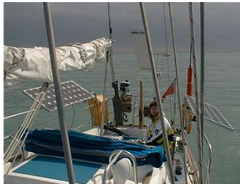
Solar panels on a small yacht to charge 12 volt batteries up to 9 amps
